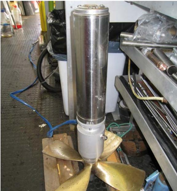
The Franklin motors are used for the main drive and for the maneuvers in all axes. A planetary gear is used in the LULA1000 to drive a large diameter propeller. This is the main propulsion unit and has the advantage that the submarine can accelerate and stop quickly. Small, directly driven propellers are used for the lateral and vertical drive.
