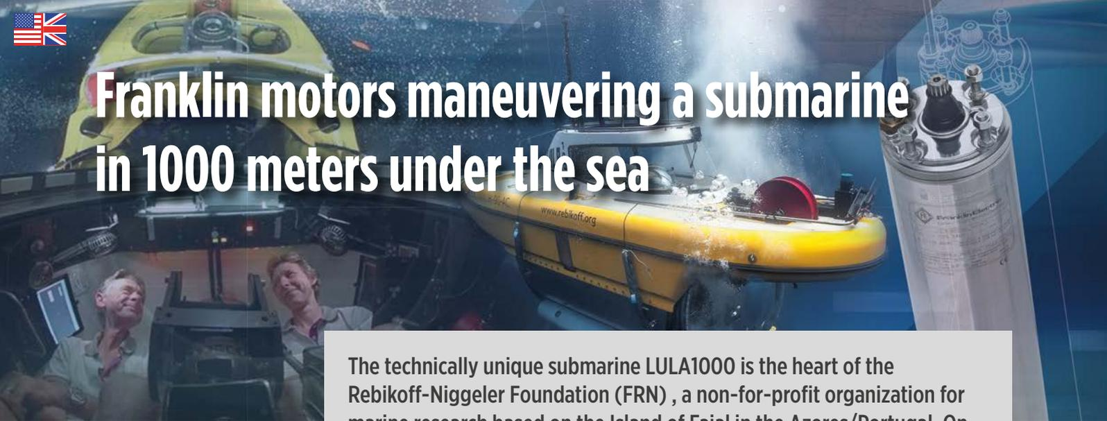
The technically unique submarine LULA1000 is the heart of the Rebikoff-Niggeler Foundation (FRN), a non-for-profit organization for marine research based on the Island of Faial in the Azores/Portugal. On board are 5 Franklin Electric 4" encapsulated motors for the main drive as well as the maneuvers in all axes.
