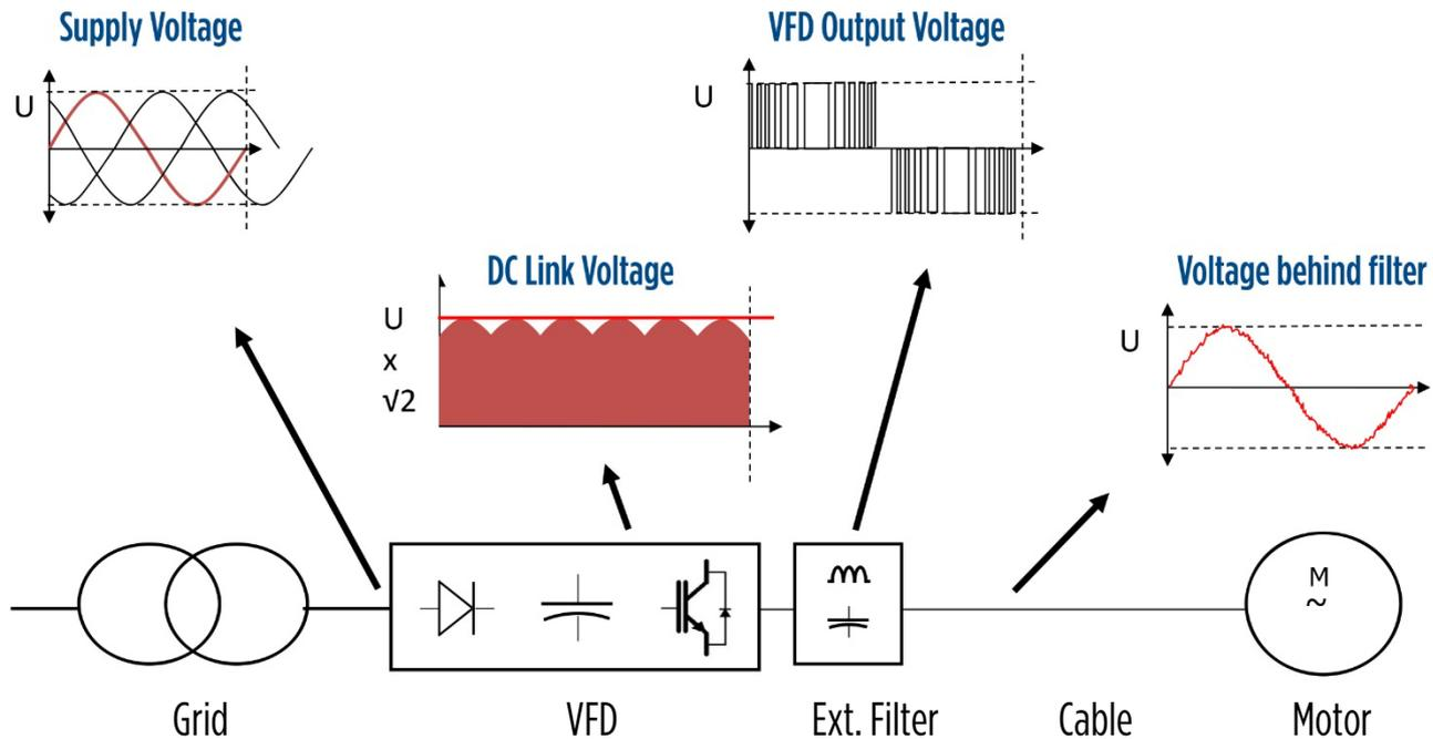
While the above is all pretty technical, what we have to walk away with is a good formula for calculating the voltage stress at the motor terminals starting from the VFD input (grid) voltage:
