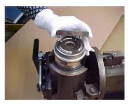
**2.** Assemble anode with supplied screws one at a time. Tighten securely with 2,2 Nm torque.
