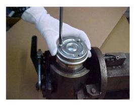
**1.** Remove one screw and washer at a time from the bottom end bell cover of the Motor.
